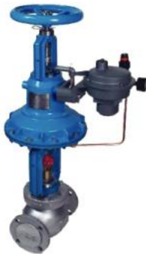
ARCA Pressure Reducing Valve 4 inch ( 100 NB) 12350 2350 Model ARCA Robotor Pneumatic Operated Input Pressu : 8.5-9 bar Output Pressure : 5-6 bar Flowrate : 6500 kg/hr
