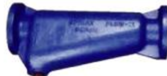
Spirax Moisture Separator 3 inch (80 NB) 4 260 1040 Body- Cast Iron- IS 210 Gr. FG260 Baffle Plate - Cast Iron -ISO 210 Gr. FG260 Ends: Flanged AS 150
